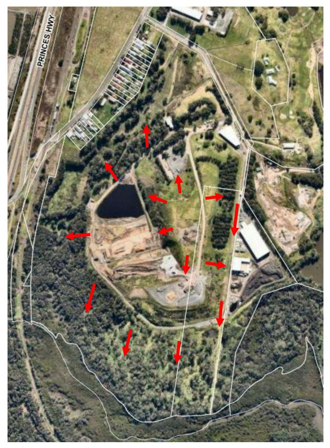
14.6 Drainage and Surface Water Flow Direction
